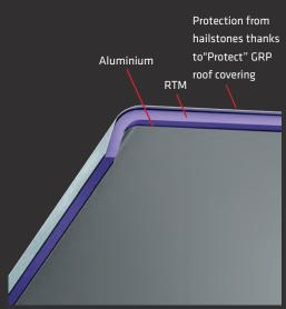
Malibu Van hybrid pop-up roof with the best insulation concept in its class in sandwich construction with light weight
